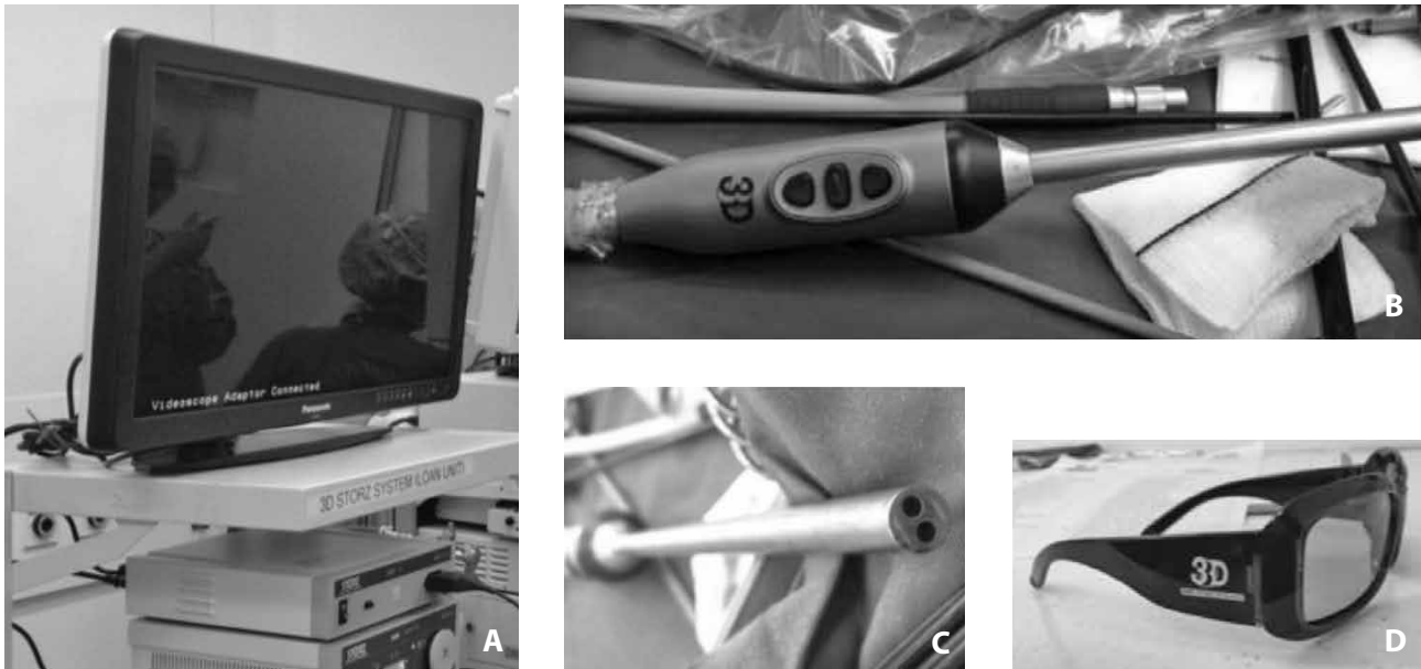
Figure 1: Karl Storz 3D Laparoscopic equipment A: 3D LCD-TV and converter; B: Telescope; C: 2x CCD chips at the tip of the scope; D: 3D glasses
